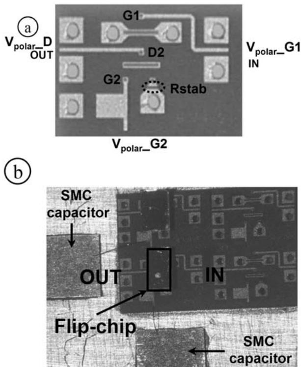
**Fig. 5.** Photograph of : (a) the AIN die designed to flip-chip the GaN cascode cell (Input and output lines, DC bias paths, Electrical bumps, Via-holes) and (b) two GaN cascode cells flip-chipped onto AIN substrate for on-wafer measurements.
