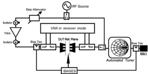
**Fig. 9.** On-wafer Pulsed Load-Pull Measurement Setup.
