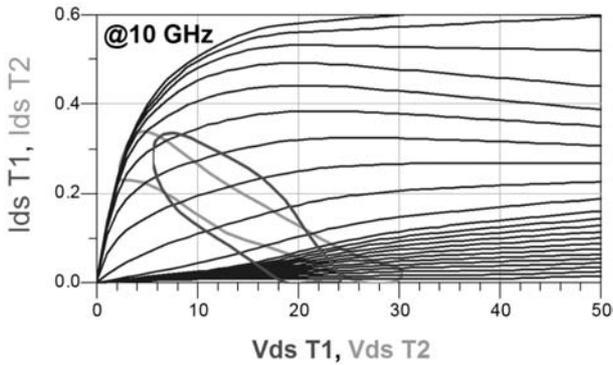
**Fig. 7.** Intrinsic load lines of each transistor of the cascode cell @ 10GHz.
