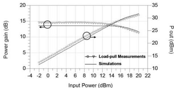
**Fig. 10.** Comparison between simulated and measured large signal results for the cascode cell @ 10GHz.
