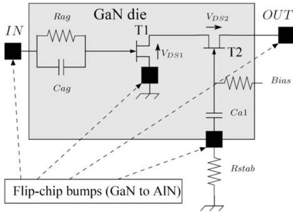
**Fig. 2.** Schematic of the power cascode cell (GaN die flip-chipped onto AlN).
