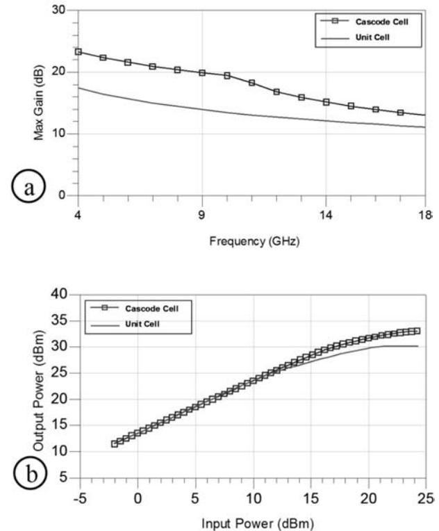
**Fig. 6.** Comparison of maximum available gain on 4-18GHz (a) and power characteristics at 10GHz (b) between the balanced cascode cell and a single transistor with input ( $Cag // Rag$ ) cell.
