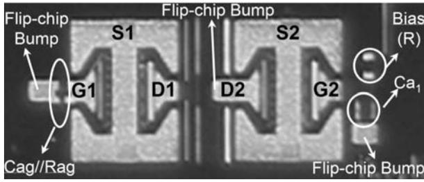
**Fig. 3.** Photograph of the GaN cascode cell.
