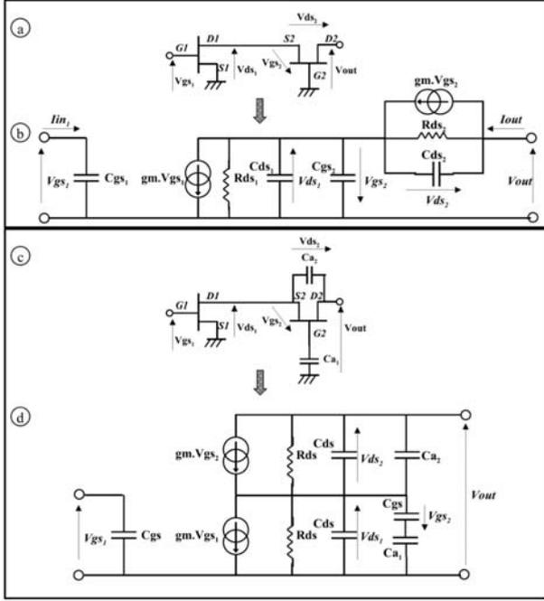
**Fig. 1.** Schematic of the theoretical cascode cell and the balanced cascode cell with the additive capacitors :  $Ca_1$  and  $Ca_2$ .
