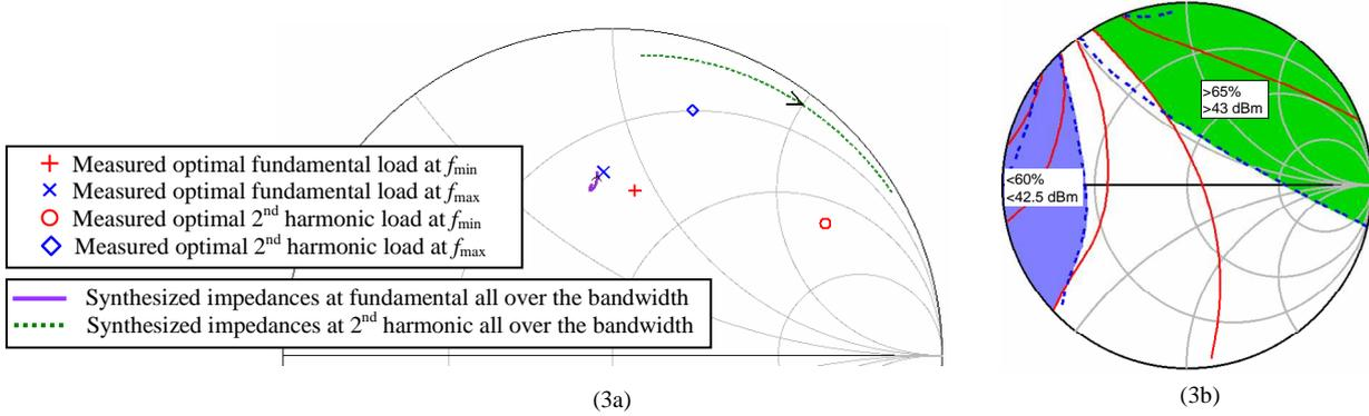
Fig. 3. Comparison of targeted synthesized and measured output loads at fundamental and 2<sup>nd</sup> harmonic over the frequency bandwidth (3.a). Simulated constant PAE and Pout circles at 2<sup>nd</sup> harmonic output ( $2x_{f_{min}}$ ) (3.b).
