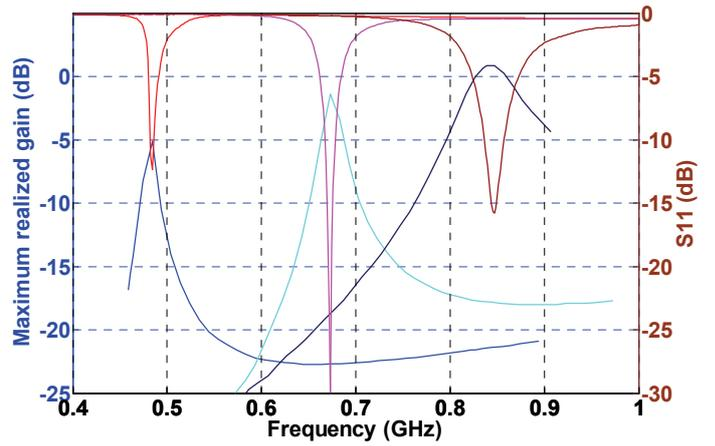
Fig. 6 Maximum realized gain and S11 for  $V=2V$ ,  $V=6V$  and  $V=22V$  polarizations of the varactor diode.
