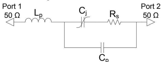
Fig. 1 Varactor diode model commonly used.
