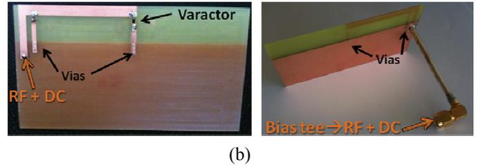
Fig. 3 (a) Design of the simulated antenna (b) Design of the measured prototype.
