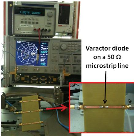
Fig. 2 Characterization of the hyperabrupt varactor diode.
