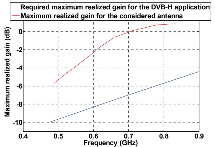
Fig. 7 Maximum realized gain on the DVB-H band.
